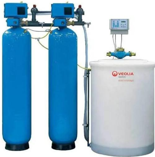
When comparing a single tank softener to a twin alternating softener, the main benefit of a single tank softener is the reduced initial investment cost, followed by slightly smaller footprint. The main benefit of a twin alternating softener is that when it is properly operating, the twin softener gives you 24/7 soft water, and is much more efficient than a single tank softener.
